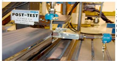
The post damage photo documentation for this October 2005 VESC V-5 test of a 1994 – 2001 Dodge Ram stepbumper to the left results in a net tow ball axis movement of 1.7 degrees as compared to the allowable Regulation movement of 5 degrees from its original, nominally vertical position.
