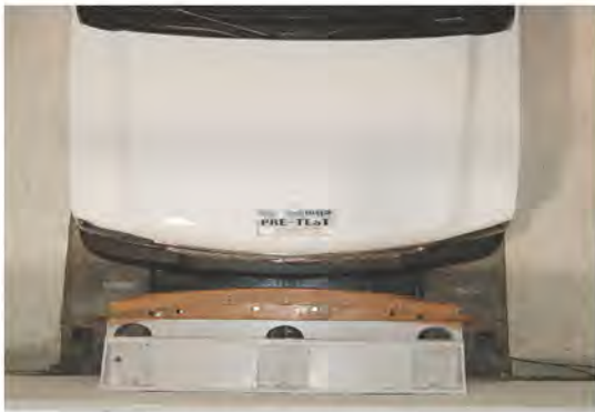
IIHS LOW SPEED CRASH TEST INTO FIXED BARRIER @ 10.0 KM/H
